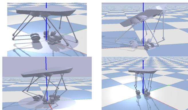
Figure: Analytical inverse kinematics solution for 6-RUS PKM.
