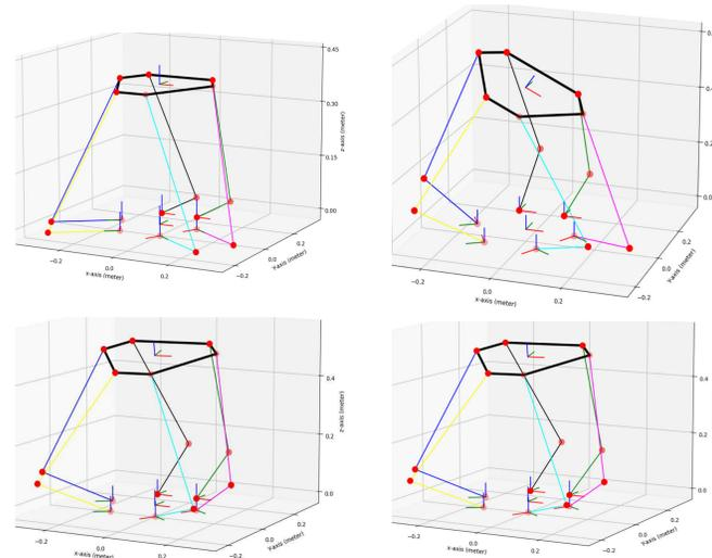
Figure: Analytical inverse kinematics solution for 6- $\overline{RUS}$  PKM.
