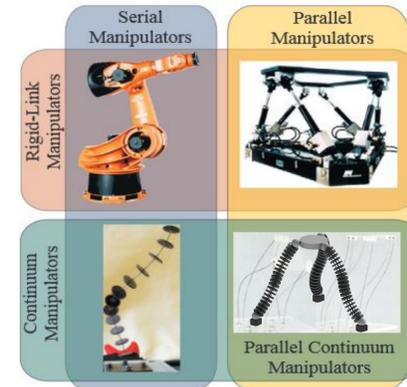
Figure: Our work aims to explore the relatively new domain of PCR situated in the 4<sup>th</sup> quadrant [1]
