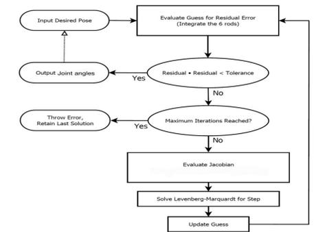
Figure: Higher level working of the solver [4]
