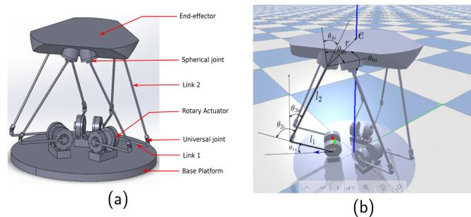
Figure: (a) The hardware setup of the proposed 6-DOF 6- $\overline{RUS}$  rigid parallel kinematic manipulator. (b) Kinematic definition for the rigid PKM
