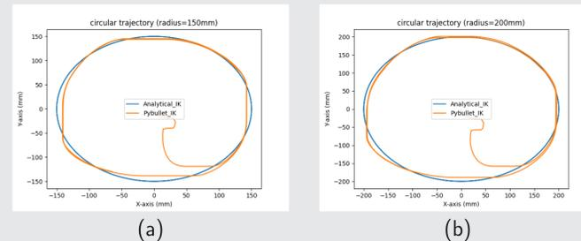
Figure: Circular trajectory comparison for (a) 0.15 radius and (b) 0.2 radius with the forward kinematic simulation using pybullet from the joint angles generated by AIK for the same circular trajectory
