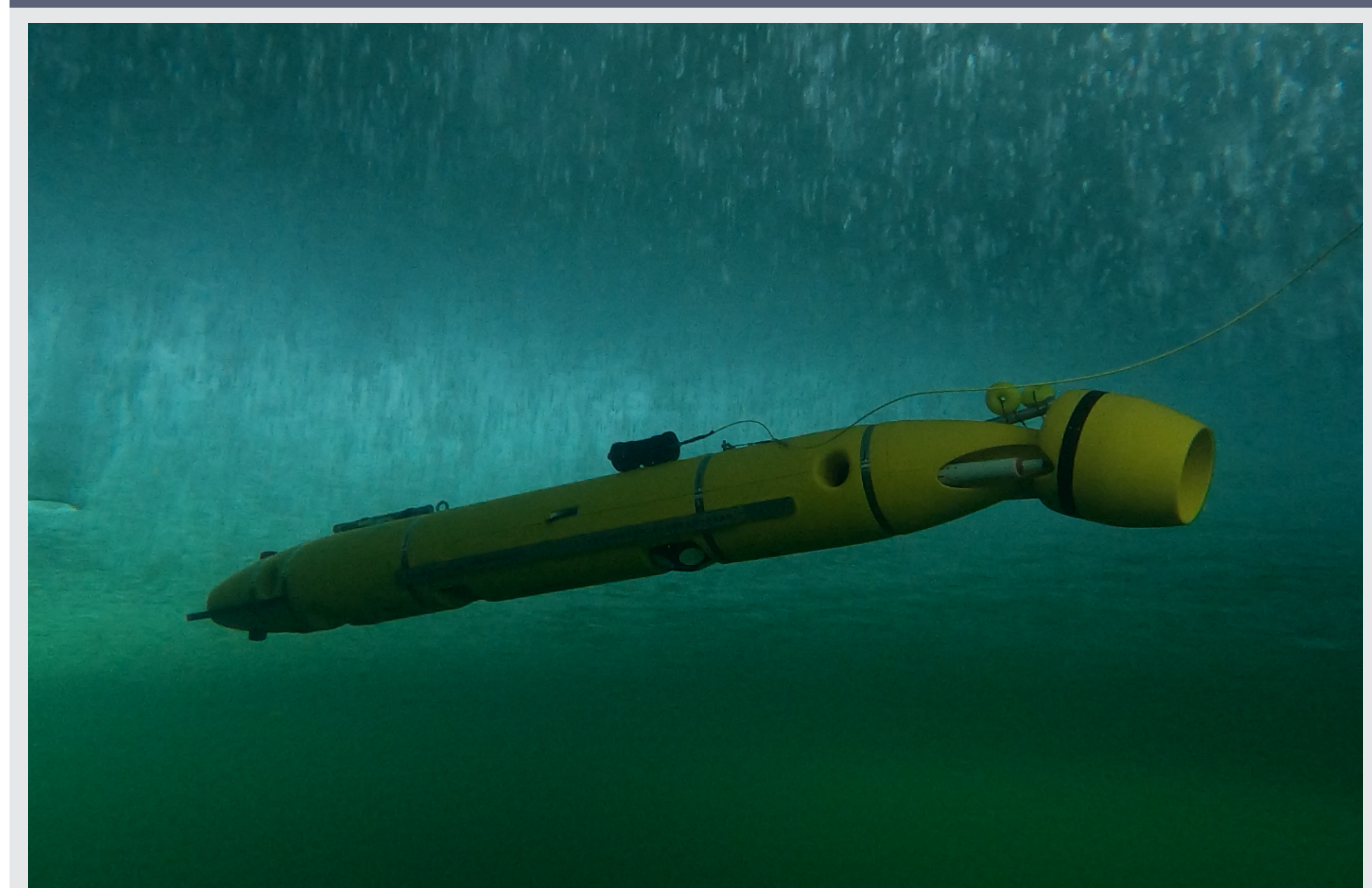
Figure: DeepLeng AUV demonstrating the vectored thrust during under-ice deployment in Abisko, Sweden [5]
