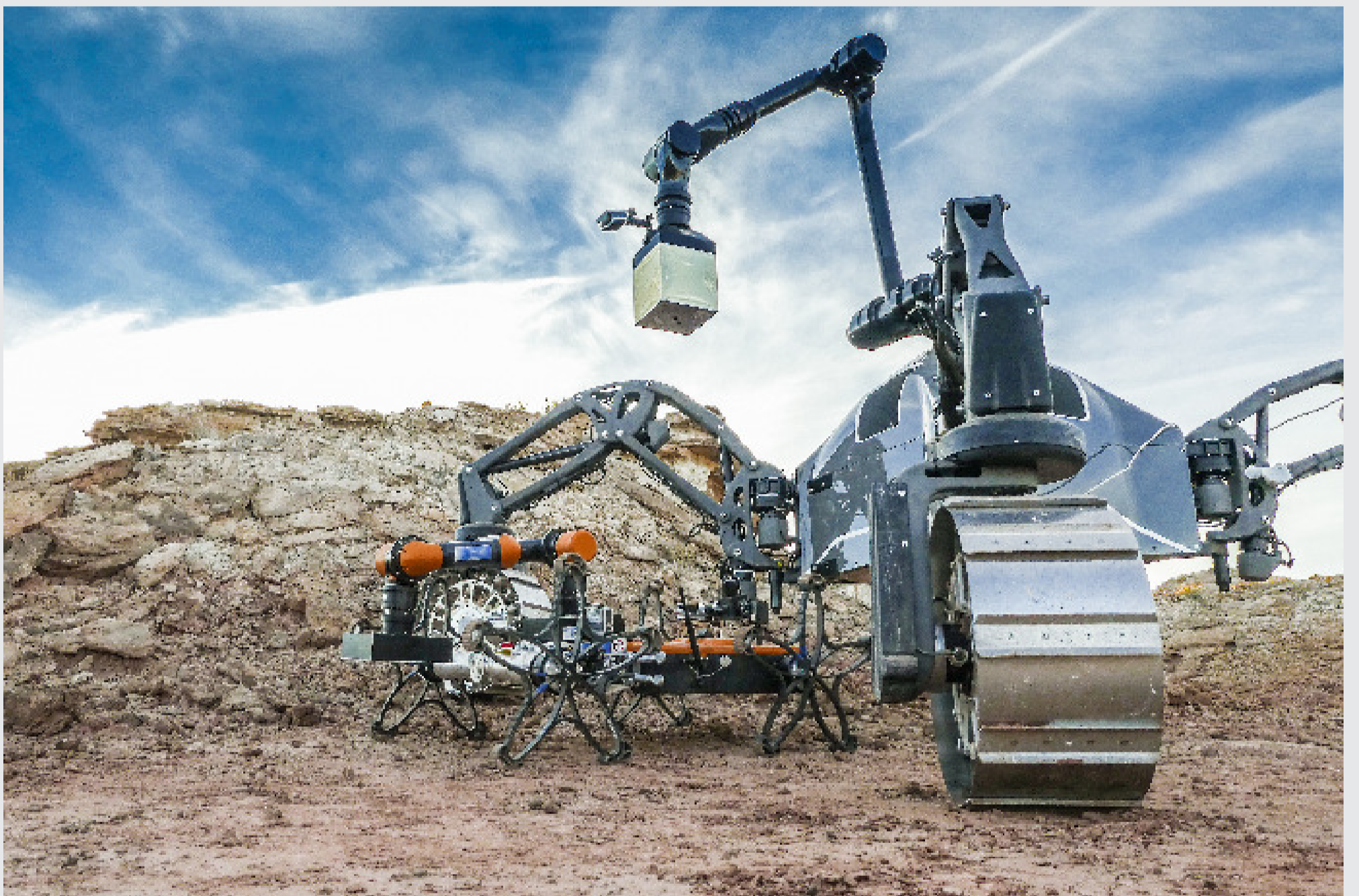
Figure: Payload exchange between SherpaTT and Coyote III in the context of the TransTerra multi-robot system [3].
