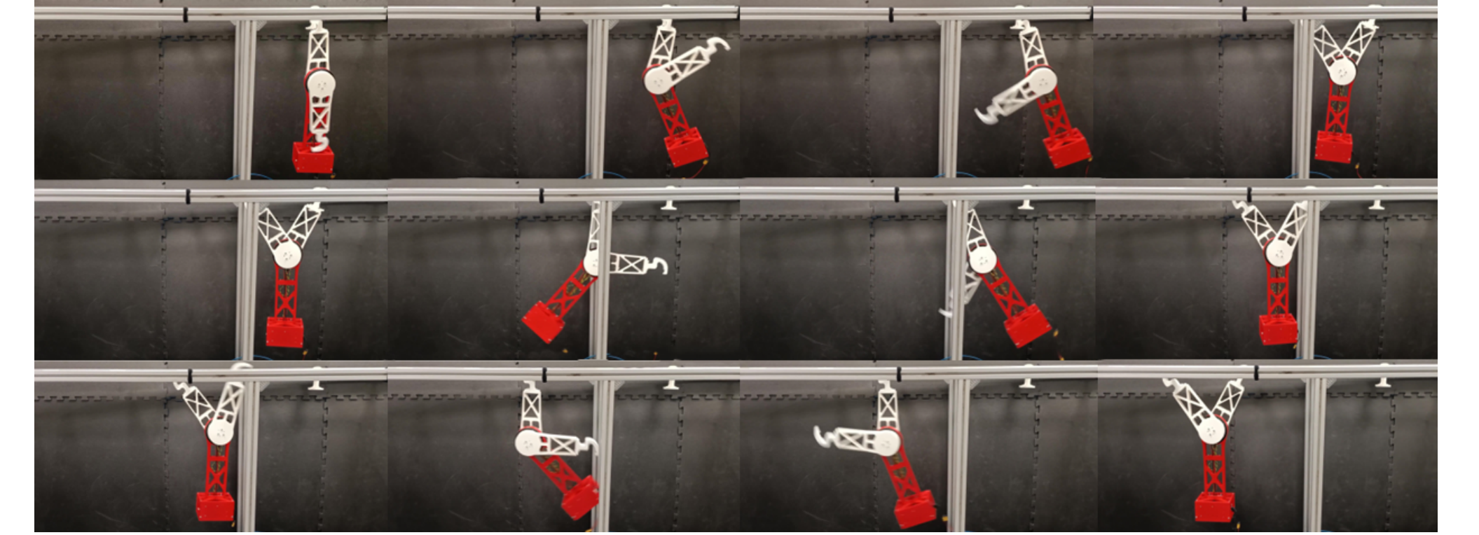
Figure: RicMonk performing multiple backward brachiation cycles. Row one - ZB maneuver (left to right), row two & three - FB maneuvers (left to right)
