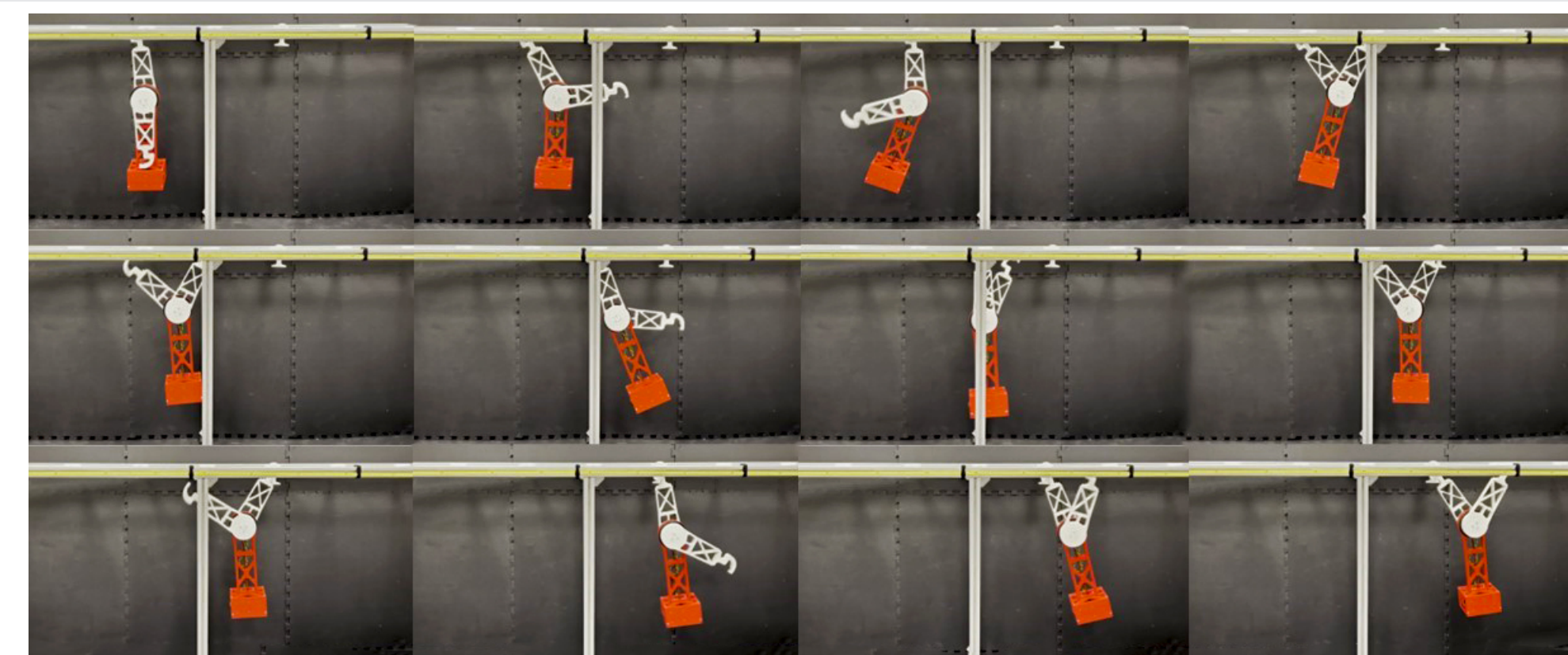
Figure: RicMonk performing multiple forward brachiation cycles. Row one - ZF maneuver (left to right), row two & three - BF maneuvers (left to right)
